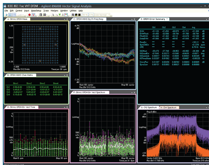
Figure 5: 89600B VSA with Option BHJ 802.11ac. Modulation Analysis supports all bandwidths and modulation types, up to 4x4 MIMO.
